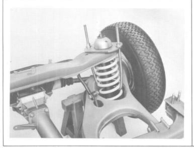
Slacken the shock absorber upper securing Nylstop nut while holding the rod with a 5 mm open ended spanner.
